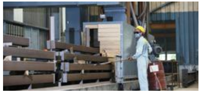
2. Surface preparation of steel by Blasting machine
